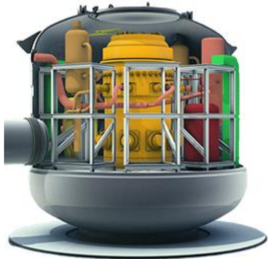
NUWARD (EdF/Technicatome), 170 MW, ab 2030
