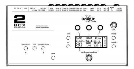
The main page comprises six logical areas. The three DATA buttons above the display are assigned to the values or functions that appear in the top row. Press the button above the desired entry to set values or select functions.
