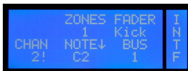
The kick drum is assigned to BUS 1
