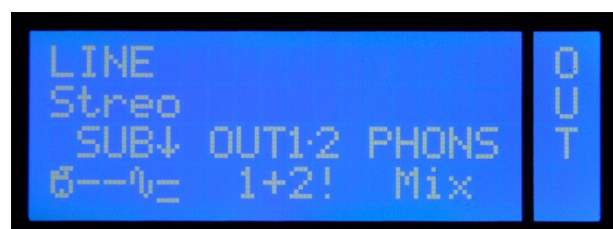
Busses 1 and 2 are assigned to OUT1 & 2
