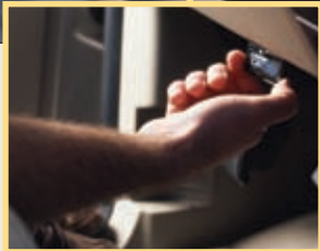
CarChip plugs instantly and unobtrusively into the OBDII port in your car or truck.
