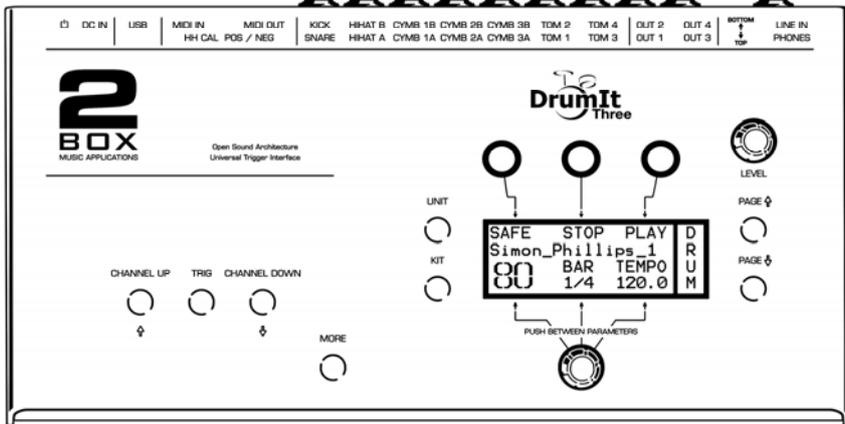
The main page comprises six logical areas. The three DATA buttons above the display are assigned to the values or functions that appear in the top row. Press the button above the desired entry to set values or select functions.
