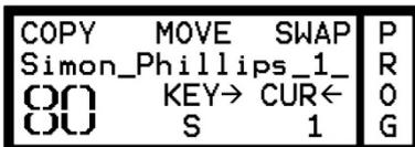
Pressing the leftmost DATA button allows you to copy the selected KIT to the target memory. MOVE allows you to move the KIT towards the target memory (the KITS at and behind this position move one slot). SWAP, finally, causes the two selected KITS to change places. In this example, KIT no. 1 moves to memory 80, while the settings of KIT no. 80 move to memory location 1.
