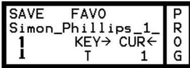
You can use uppercase and lowercase letters, numbers as well as several special characters for the names you enter. Use the knob to select the desired character (KEY flashes) or hold down the MORE button while pressing the knob to insert a space. Press the knob without holding down the MORE button to select the CUR parameter. Now, the knob can be used to move the flashing underline cursor to another position you want to edit.
